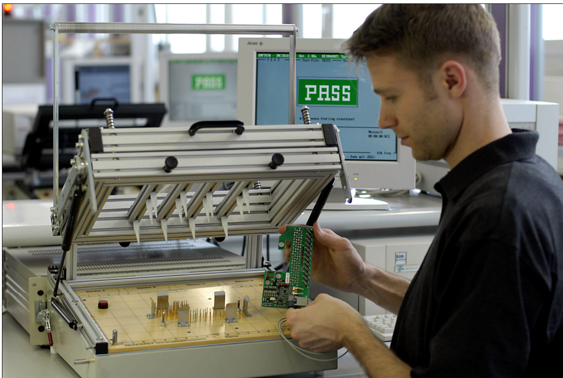
Fig. 6: Integrated in-circuit and functional tests with automated test equipment (ATE)
